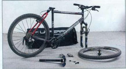
Packing: Putting the Passport into its cocoon is close to a tool-less endeavor. Removing the pedals was the only step when we had to use a tool (an Allen key from the supplied multi-tool).
