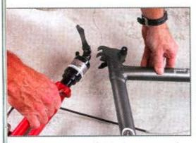
Quick tricks: Quick releases are used on the seatstays/shock (shown), the seatpost and the handlebar stem. The bar does not need to be removed from the stem for packing. That saves a ton of time.
