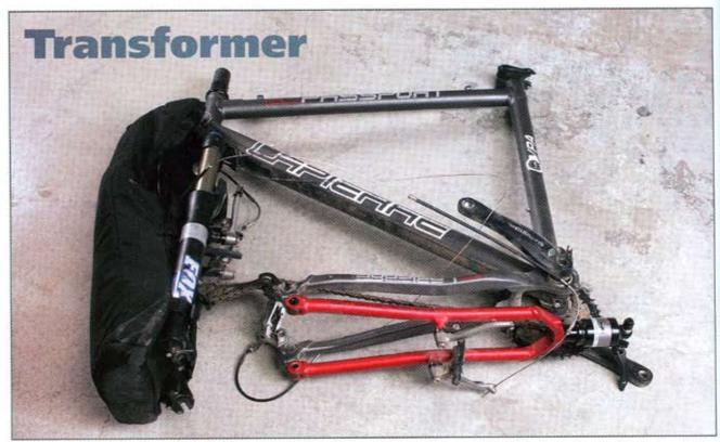
Compact Passport: The bar and stem are tucked in a bag and strapped to the reversed fork. The seatstays and chainstays fold under the downtube, and the low-normal rear derailleur tucks in perfectly between the fork sliders.
